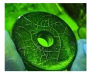
ZChek Magnetic particle inspection materials confirm to specifications of
