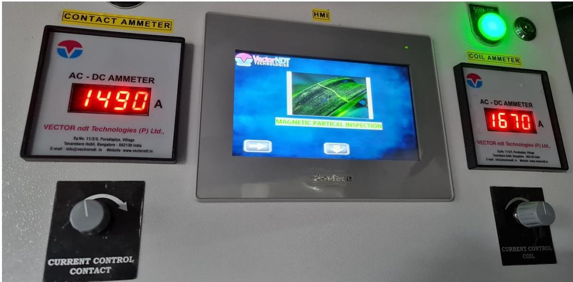
Digital Ammeters with memory retention – will retain the reading till the next magnetizing shot
