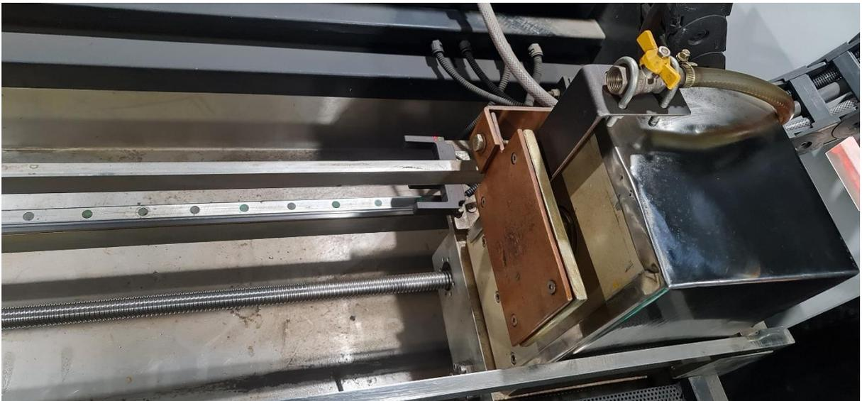
Optional Servo driven Magnetizing Coil for automatic multiple coil shots
